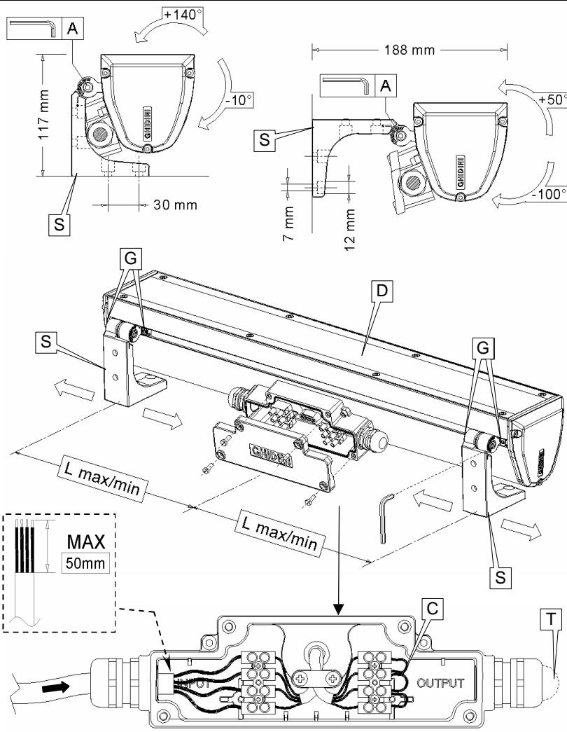
Fix the lighting unit to the bearing surface (wall, frame, pavement or ceiling), to suit your needs, with the two pre-assembled brackets (S) with 4 - Ø6 screws (NOT supplied).
